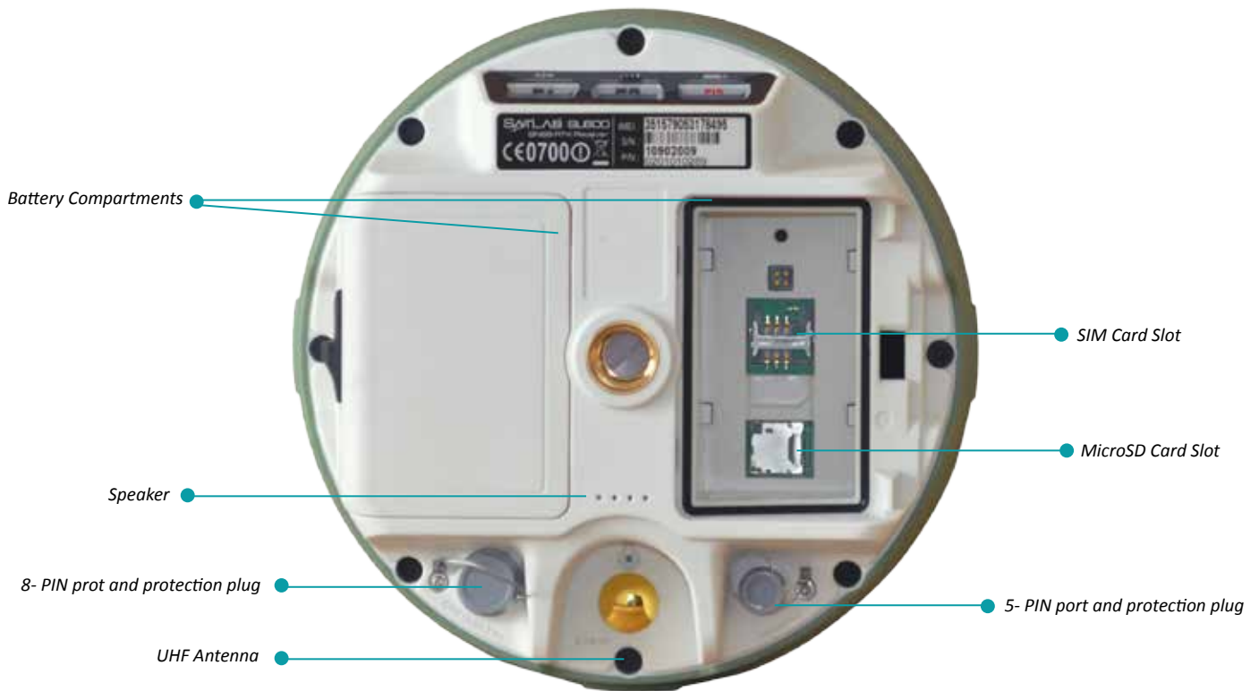
Figure 2.3 shows the components of bottom part.
